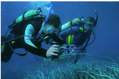
The diver holds the SeaSlate by its two grips (with elbows resting on the side wings) so that the screen (which is in "portrait" mode) is immediately in the field of view. Field trials have shown that the computer can be steered using one hand and be easily operated (even using gloves) whilst swimming.
